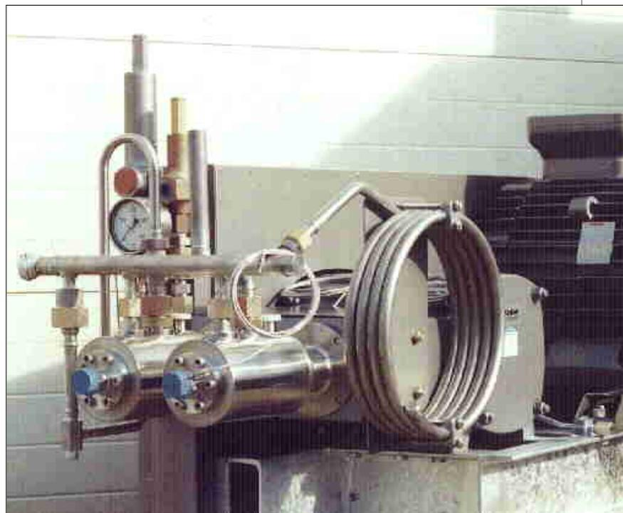
*Twin head TLC-pump, explosion proof construction for LNG;
