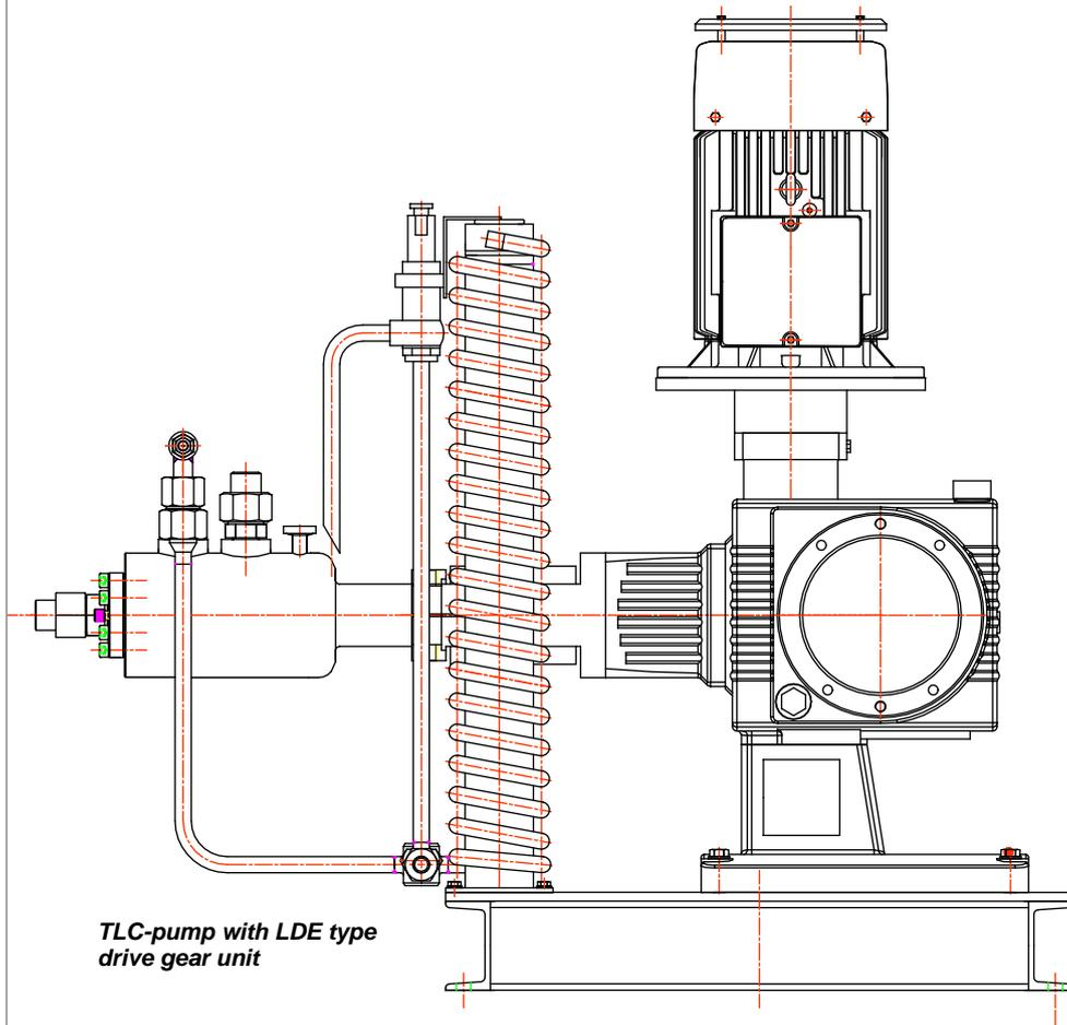
*TLC-pump with LDE type drive gear unit*
