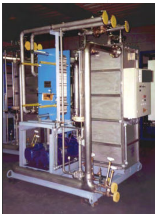
PAREX evaporator for N 2 / O 2 : 2000 / 4000 Nm 3 /h; district heating via secondary circuit
