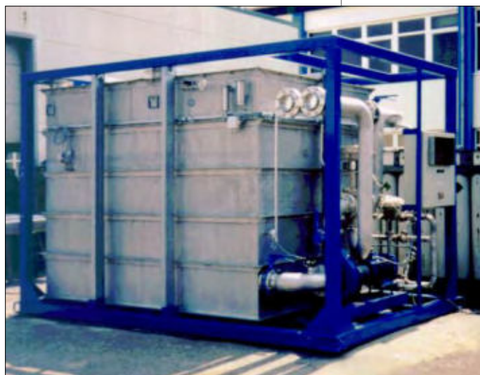
PAREX-evaporator for power station emergency supply: 18000 Nm 3 /h O 2 + 5000 Nm 3 /h CH 4 heat transfer medium: cooling water 50°C
