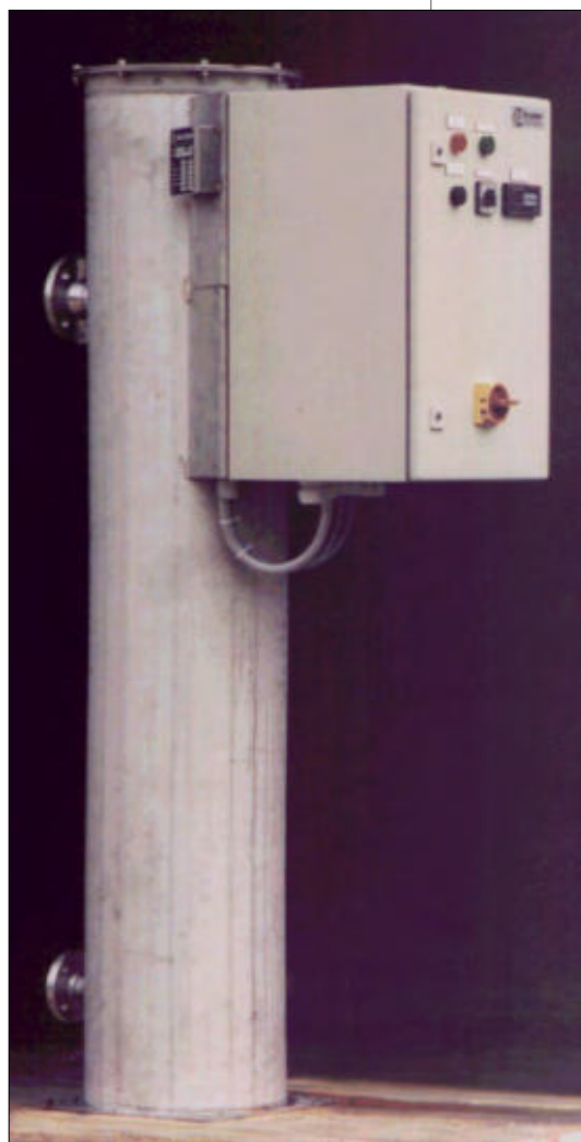
CENTREX gas heater with thyristor control: O_2 post heating approx. 1000 \text{ Nm}^3/\text{h} ; \Delta\theta \approx 50^{\circ}\text{C} ; outlet temperature +25 \pm 1^{\circ}\text{C}
